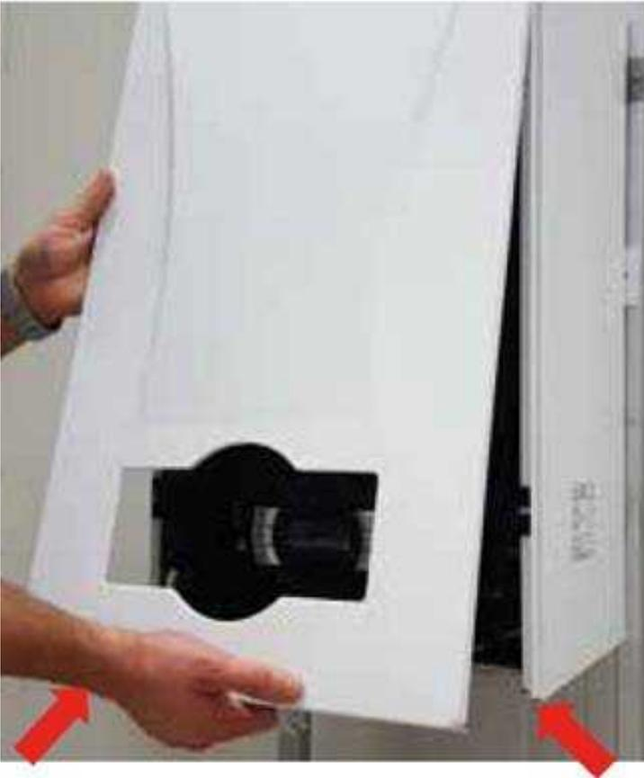
Dismounting Side Panel: Unscrew 2 screws affixing the control panel to the side panels.
