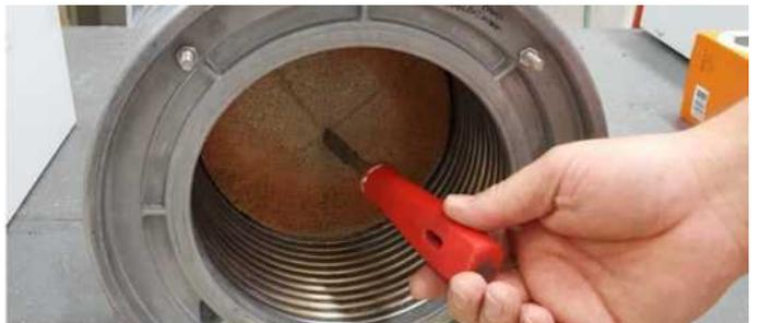
➤ Remove 4 screws of the burner door. Follow the order of operations (shown as wrench symbol) inscribed on the burner door when dismantling and remounting.
