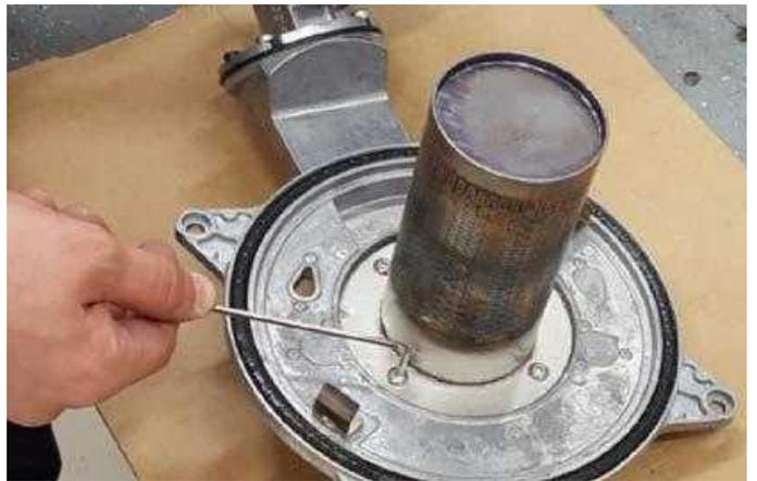
➤ Remove 4 nuts fastening the burner and the cover using an Allen tool.
