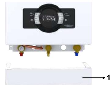
Figure 9. Isolation Valve Cover Mounting
